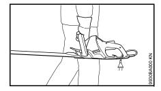
Carry the machine by the handle – with the cutting blades pointing to the rear.
